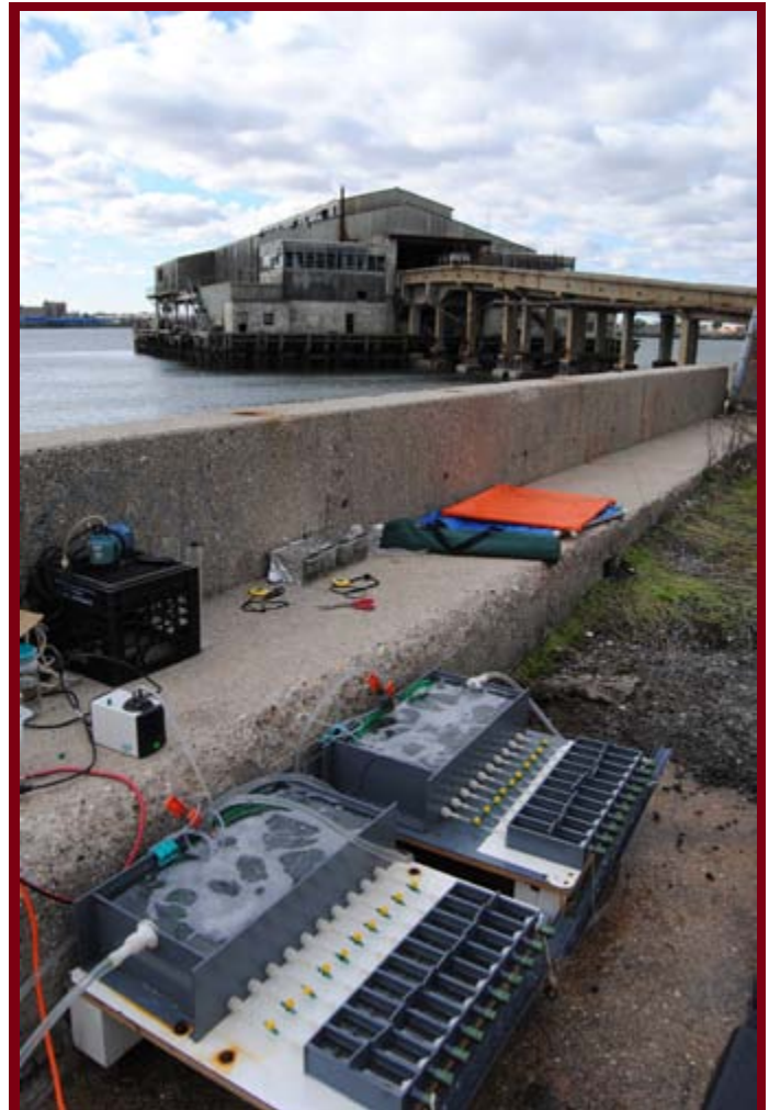
Apparatus to measure mussel filtration at the Bronx River field site. An abandoned waste transfer station is visible in the background. Local water is pumped through the system and across individual mussels, and their feeding activity is measured within each chamber.
