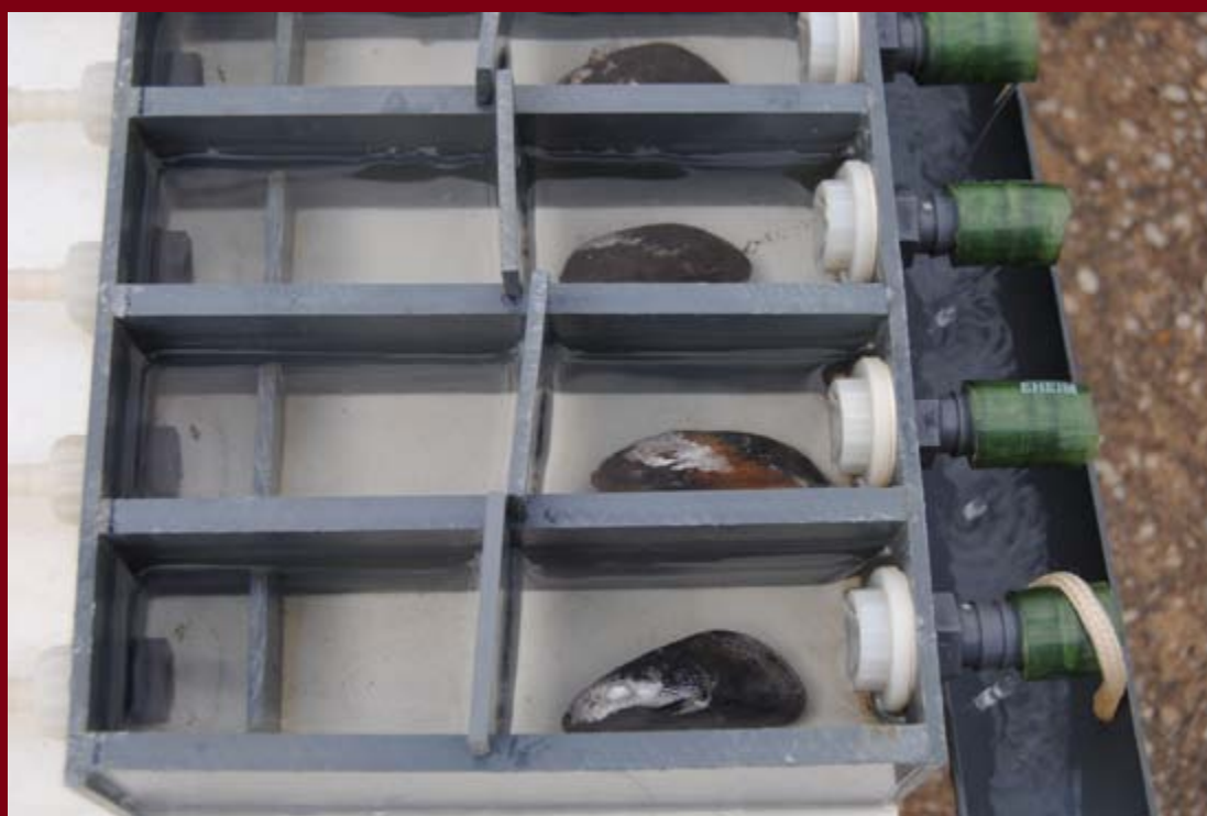
Ribbed mussels inside chambers of the filtration apparatus. Local water is pumped in from the left, then flows directly across each mussel before exiting the chamber on the right. (Credits: Larissa Graham, New York Sea Grant Outreach Coordinator, Long Island Sound Study)
